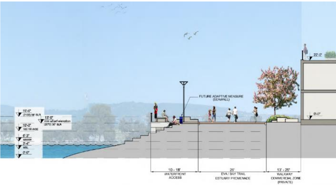
FIGURE 2.7 ADAPTIVE MEASURE AT NORTHERN ESTUARY EDGE, IN WATERFRONT PARK, SECTION P6
